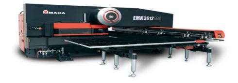
The 3612 Processes 10'x5' sheets without repositioning, the highest real-world hit rates and ram positioning accuracy. Precision ram motion control (speed, stroke length, hover height and hold time) Standard 58-station triple track, King turret.
